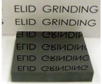
Fig. 6: ELID Grinded Test Piece
