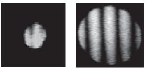
Fig 6 : Impact on the fringe contrast versus the diffuser position for tilt. In the left image the diffuser is at 100 mm from the best focus once for the right image it is at 300 mm.
