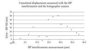
Fig 5 : Holographic camera calibration with a commercial interferometer of displacement of several tenth of  $\mu$ m.
