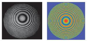
Fig 4 : Interferograms of the spherical mirror defocused observed by the holographic camera using an intermediary diffuser (left) and simulated (right)
