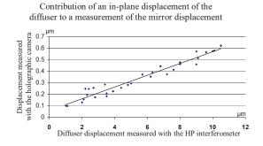
Fig 7 : Contribution of diffusers displacement in plane to the measured displacement of the mirror.
