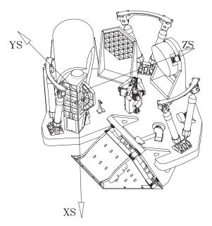
Fig. 9 : overall mechanical layout of the LIFT instrument
