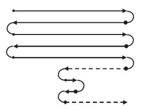
Fig. 5 :Interferogram mechanism movement during acquisition and calibration
