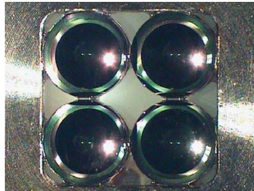
Figure 21 : microlenses support (front face)
