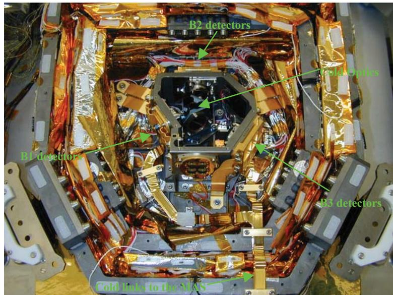
Fig. 1. Detectors integrated in Cold Box
