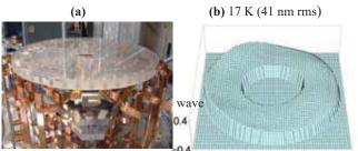
Fig.10. (a) Reflecting flat mirror mounted on the stage inside the chamber. (b) Cryogenic deformation of the flat mirror.
