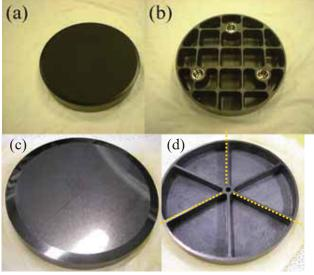
Fig.2. (a) 160-mm-diameter SiC mirror and (b) its rear-side structure. (c) 160-mm-diamter C/SiC composite mirror, and (d) its rear-side structure.
