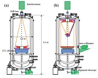
Fig.4. Schematic views of optical measurements of (a) primary mirror, and (b) telescope assembly.
