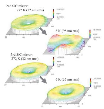
Fig.6. Changes of surface figures for the second (upper) and the third SiC mirror (lower) with temperature.
