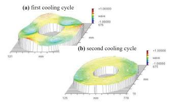
Fig.8. Difference in surface figure of the primary mirror between before and after (a) the first cooling cycle and (b) the second cooling cycle.
