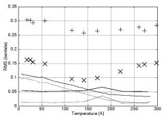
Fig.11. Plots of surface figure error for the C/SiC composite mirror against temperature (pluses). Figure error relative to the initial surface figure measured before the cooling is also plotted (crosses). In addition, figure errors for the second and the third 160-mm SiC mirror are shown in a dotted and a solid line, respectively.
