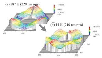
Fig.9. Changes of surface figure (half the total wavefront error) for the telescope assembly with temperature.
