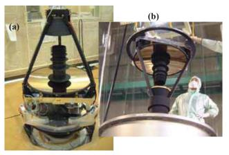
Fig.5. ASTRO-F flight-model telescope during (a) vibration test and (b) installation into the chamber.
