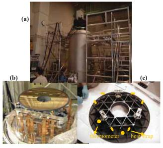
Fig.1. (a) Test chamber facility, (b) ASTRO-F primary mirror mounted on the cold stage inside the chamber, (c) rear-side structure of the primary mirror.
