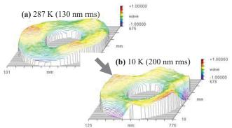
Fig.7. Changes of surface figure for the primary mirror with temperature. Both are shown in the same scale.
