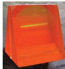
Fig. 7 ZnSe VPH grism for FOCAS with very high dispersion ( $R=7,000$ ).
