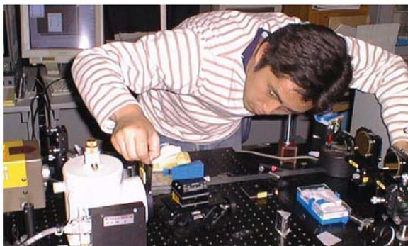
Fig. 15 Measurement of far-field image of immersion grating.
