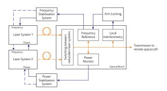
Figure 2. Frequency and power stabilization scheme.
