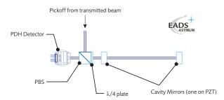
Figure 3. Typical setup for frequency stabilization to a cavity reference. The setup would be installed together with all interferometers on the optical bench. It would thus profit from the high dimensional stability provided by the Zerodur baseplate and the exceptional temperature stability of  $10^{-5} K/\sqrt{Hz}$ .
