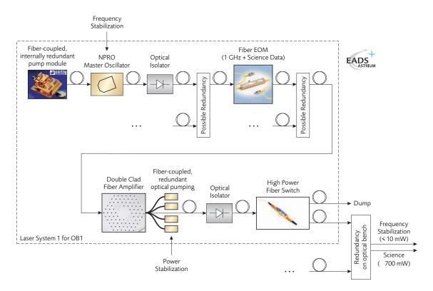
Figure 1. Overview of a possible MOFPA laser system for LISA. For concreteness, the schematic assumes the use of a low power diode pump module by TESAT for the master oscillator, a LiNbO<sub>3</sub> broadband waveguide EOM by Guided Color Technologies GmbH, and a NanoSpeed High Power  $1 \times 2$  Solid-State Fiberoptic PM Switch by Agiltron.
