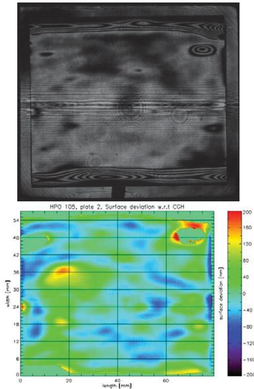
**Fig. 3-1:** Above, interferogram w.r.t. to a CGH, recorded at wavelength 633 nm, on the 2<sup>nd</sup> silicon plate that is stacked onto a Zeiss polished mandrel, which is larger than the plate and also visible. Central horizontal lines are artefacts caused by the CGH. Bottom image shows surface deviation of the same plate w.r.t. the mandrel. 80% of the area is fully bonded and within one fringe. Cylindrical axis is horizontal.
