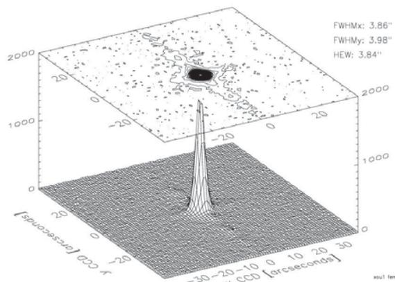
**Fig. 3-4:** First recorded reflection of an x-ray beam imaged by a silicon pore optic, integrated and fixed in Wolter-I configuration<sup>10</sup>.
