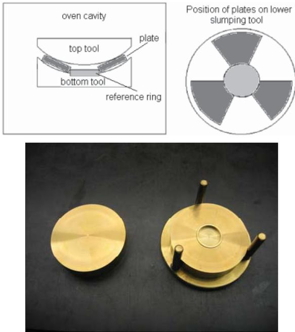
Fig. 2-3: Schematic of radial plate positions in the slumping mould and photo of the mould used.
