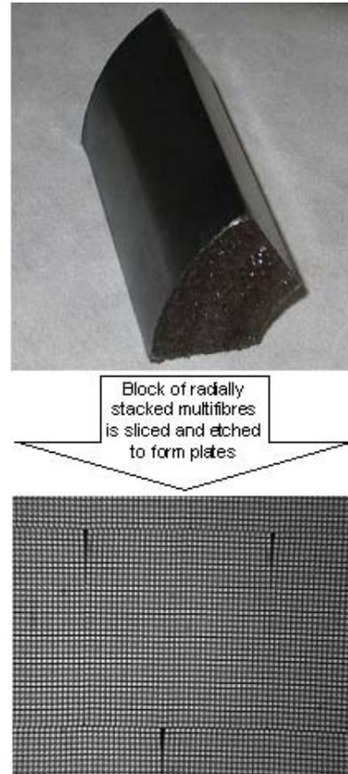
Fig. 2-2: Fused block of radially stacked micro-pore material above. Microscope image of sliced & etched plate below, one MF visible with surrounding MFs
