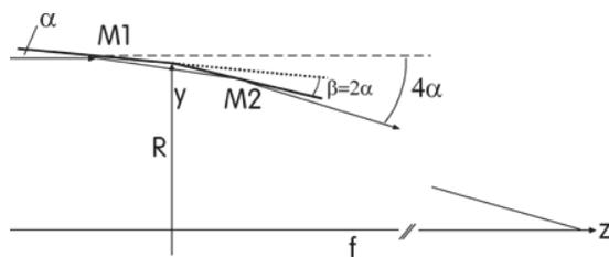
**Fig. 3-3:** Schematic of the Wolter-I configuration. M1 is parabolic, M2 hyperbolic.  $R$  = radius and  $f$  = focal length. X-rays enter from the left side. Petal is in the  $x/y$  plane.
