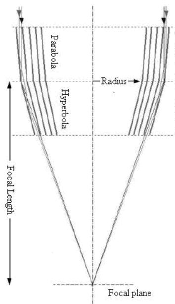
Fig. 1-1: Conical approximation of the parabolic and hyperbolic sections of a Wolter I optic to focus x-rays.
