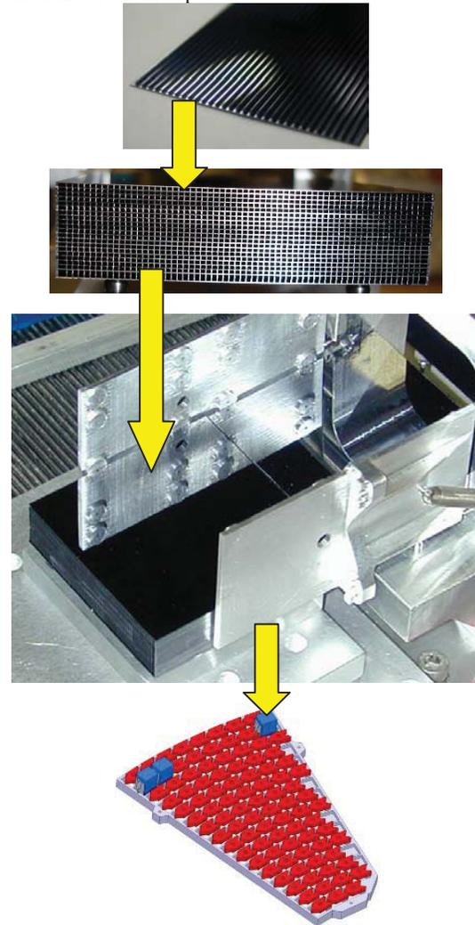
**Fig. 3-2:** Integration concept of silicon pore optics. Ribbed silicon plates (top) are bent and assembled on a mandrel to form porous structures. Two plate stacks are co-aligned and integrated using brackets to form a Wolter-I x-ray lens. Tens of tandems are then integrated into a petal structure (bottom).
