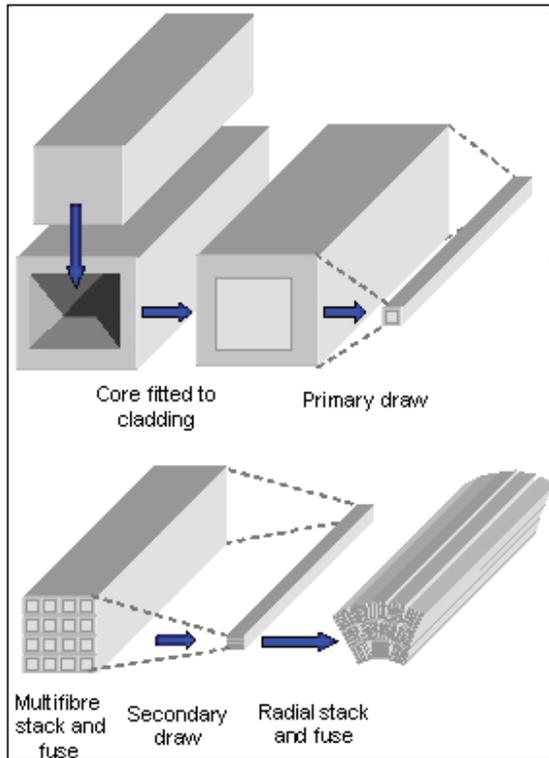
Fig. 2-1: Manufacturing steps to produce MCP material
