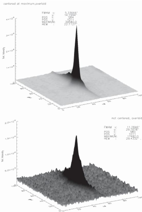
Fig. 2-4: Results of tests with a 3keV,  $100\mu\text{m}$  pencil beam
