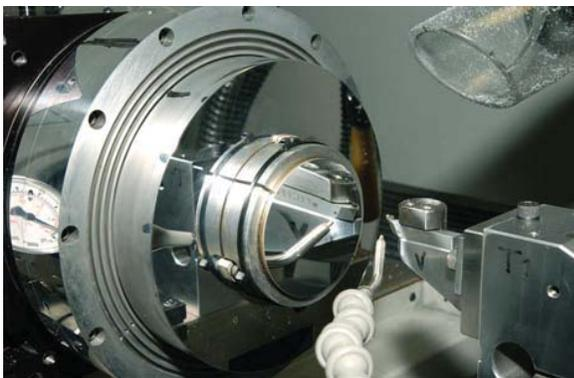
Fig. 2 - Diamond turning of M1 mirror
