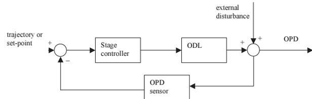
Fig. 5. OPD control model of single stage delay line
