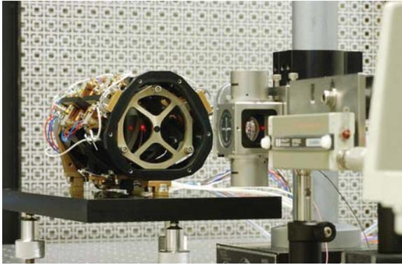
Figure 6 – ODL with laser interferometer
