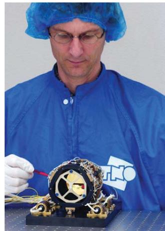
Fig. 1 - Darwin Breadboard Optical Delay Line
