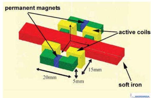
Fig. 3 - Active magnetic bearing
