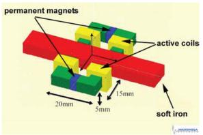
Fig. 3 - Active magnetic bearing
