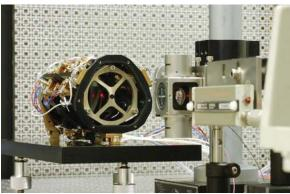
Figure 6 – ODL with laser interferometer
