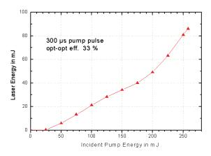
*Fig. 3: Performance of the longitudinally pumped laser at 942 nm wavelength: Output versus input energy of Nd:GSAG*
