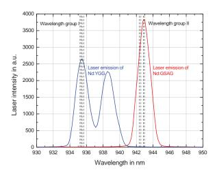
*Fig. 1: Spectra of Nd:YGG and Nd:GSAG laser emission covering water vapor absorption lines*
