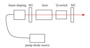
Fig. 2: Laser setup longitudinally pumped from one side with up to 300 mJ pump energy in 300  $\mu$ s pulses at 1 kW peak pump power
