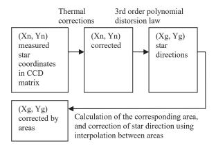
Fig. 3. Flight software distortion correction process.
