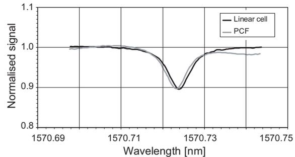
Fig. 12. Normalized transmission through a 1-m linear cell and a 1-m HC-PCF, both filled with CO<sub>2</sub> at reduced pressure (100 mbar). The wavelength was scanned by current tuning a DFB laser. Amplitude and width of the absorption lines are identical. The slight wavelength shift between the two measurements is due to the precision and operation repeatability of the laser temperature control.
