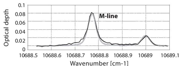
Fig. 7. Comparison of calculated (bold grey line) and experimentally measured (black thin line) absorption line for the medium strength line  $\lambda_2$  (left-hand) using FRU2. For this line, the calculated data for the optical depth peak value and linewidth are 0.077 and 1.20 GHz, while 0.083 and 1.28 GHz were retrieved from the experimental fitted data.
