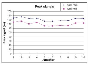
Fig. 8. Charge capacity
