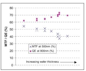
Fig. 6. MTF and QE trade-off vs thickness
