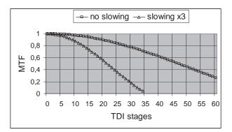
Fig. 2. Loss of MTF due to registration discrepancy-PLEIADES-HR case
