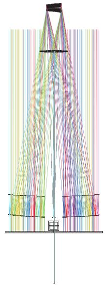
Fig.3 Baseline optical design – view on XZ plane
