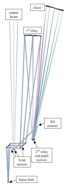
Fig. 2 Baseline optical design – view on YZ plane
