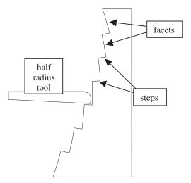
Fig. 6 Slicer schematic: cutting problem
