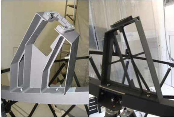
Fig. 8. Ultralightweight brackets for X- and S-band antenna on top of external baffle
