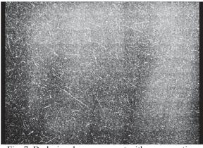
Fig. 7. Dark signal measurement with exposure time 136 seconds and gain factor 40 in South Atlantic Anomaly (SAA). The increased number of random hits and trails of particles can be observed.
