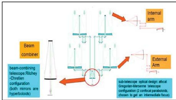
Fig. 1: interferometer optical design
