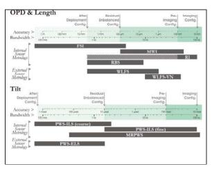
Fig. 7. Sensors for OPD and length measurements (top) and tilt measurement (bottom).
