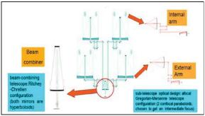
Fig. 1: interferometer optical design
