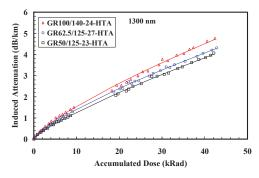
Fig. 3. γ-radiation data of MM fibers at 1300 nm.
