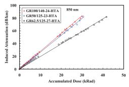
Fig. 2. γ-radiation data of MM fibers at 850 nm.
