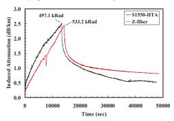
Fig. 5. Proton test data of S1550-HTA fiber.
