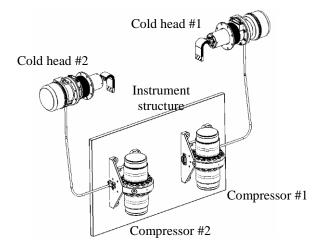
Fig. 4. MPTC redundant architecture integration
