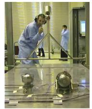
Fig. 9. LPTC S/N001 during shock test.
