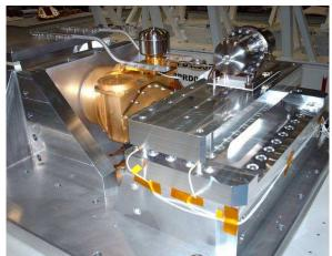
Fig. 11. EQM LPTC S/N002 integrated on a cryostat mock-up (courtesy of ThalesAlenia Space)
