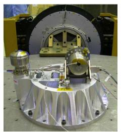
Fig. 5. EM S/N001 installed on the shaker
