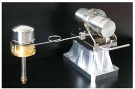
Fig. 1. EQM MPTC cold finger and compressor
