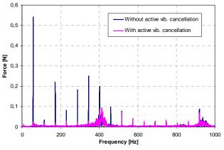
Fig. 12. EQM LPTC S/N002 self induced forces at compressor interface – 160 Wac input – 50K
