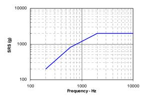
Fig. 8. shock load qualification profile
