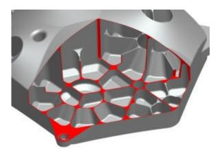
Fig. 8. Inside rib distribution of extreme lightweighted study model based on the X-Shooter M7.
