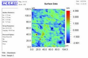
Fig. 2. Polished sample, Ra= 0.59 nm
