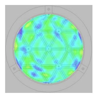
Fig. 6. Residual irregularities of the 300 mm M7 layered on a mechanical drawing of the back of the mirror. The relation between light weight pockets and print through is visible but insignificant: Residual irregularities are in the range of 4nm RMS, while surface roughness is still around 1 nm (Ra). The OPD map (created with Intelliwave) shows the remaining irregularities, with tilt, focus, astigmatism, symmetric and asymmetric subtracted.
