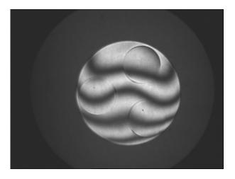
Fig. 3. Fringe pattern of the concave 200mm mirror after polishing (three segments visible).
