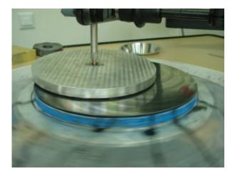
Fig. 4. M7 during a polishing session, mirror face up. The polishing tool on top has a 5 mm thick layer of specially prepared polishing pitch.
