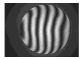
Fig. 5. Fringe pattern of M7 after p olishing, showing less than 1 fringe surface error over the entire 300 mm diameter
