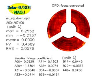
Fig. 4. The wavefront error map of the OTA for the zero-gravity condition.
