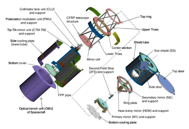
Fig. 2. Layout of the OTA structural assembly.
