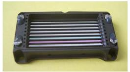
Fig. 3: VNIR Filter Assembly
