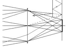
Fig. 1(d). Trapping of  $\underline{r}$  and rejection of a ray entering parallel to  $\underline{r}$  (on the top)
