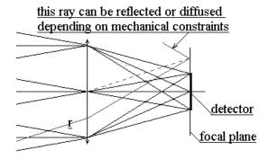
Fig. 1(a). First order ray tracing layout of the spatial filtering concept. The skew ray  $\underline{r}$  is reflected by a flat focal plane.
