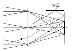
Fig. 1(b). First order ray tracing layout of the ray  $\underline{r}$  reflected by a lateral wall after reflection on the insensitive area of the detector.
