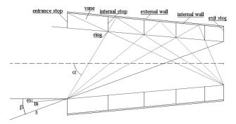
Fig. 2. A typical baffle design
