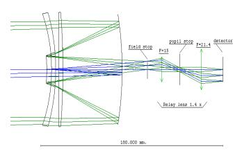
Fig. 4. Overall layout with a first order relay.
