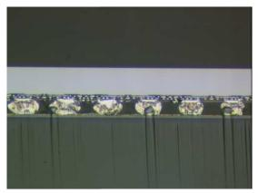
Fig. 12: SEM image of a polished readout circuit hybridized to an AlGaN on sapphire 2D array.
