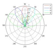
Fig. 3.-Theoretical radiation diagrams of an array of 4 antennas placed behind the beamforming unit.
