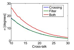
Fig.5 Standard deviation from the ideal phase distribution due to the interference generated at the crossing and filters of the structure.
