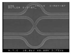
Fig. 2.- SEM Image of the 4x4 Photonic Butler Matrix
