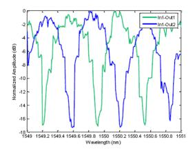
Fig. 4.-Normalized transmission of the MZI structures used to separate the CW components of the heterodyne signal.
