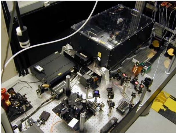
**Fig. 3.** The Adaptive Nuller Testbed (AdN). The Adaptive Nuller demonstrated phase and intensity compensation of beams within a nulling interferometer to a level of 0.12% rms in intensity and less than 5 nm rms in phase. This version of the AdN operates over a wavelength range of 8–12  $\mu\text{m}$ . The long-focus parabolas, used in AdN are seen on the upper right.
