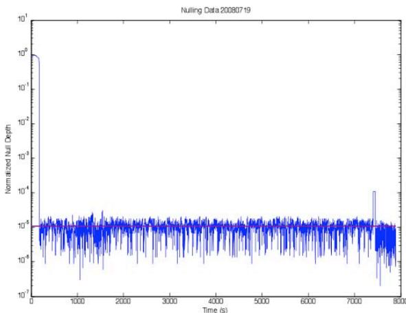
**Fig. 4.** Results from the Adaptive Nuller testbed show stable nulls at a level of 93,000:1 over a period of two hours. A bandwidth of 32% was used centered on 10  $\mu\text{m}$ .
