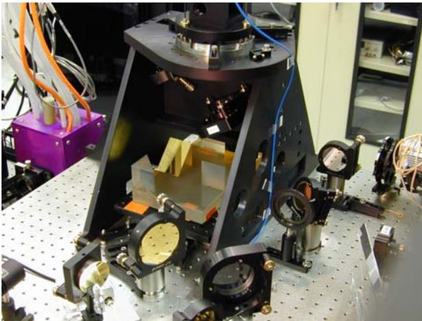
**Fig. 2.** View of the periscope assembly of the Achromatic Nulling Testbed.
