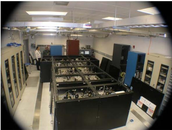
**Fig. 5.** The Planet Detection Testbed (PDT). The PDT is a four-input nulling interferometer that uses  $10\ \mu\text{m}$  laser light and servo loops to perform experiments related to instability noise, interferometric chopping, and planet detection. The testbed configuration shown here has obtained laser nulls between 500,000:1 and 800,000:1 and detected a simulated planet with a contrast ratio of 2,000,000:1.
