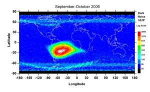
Fig. 12 Dark noise map for the 532 parallel channel
