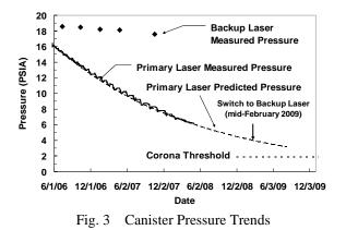
As of September 2008 the primary laser pressure is approximately 5 PSIA. At this level, low pressure is causing no problems, but there is a potential for a corona discharge due to the high voltage within the canister if the laser operation is continued to below about 1.9 PSIA. A switch to the backup laser is currently planned for mid February 2009, well before the pressure reaches the corona threshold.
