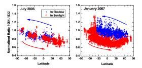
Fig. 9 Normalized channel ratio (1064 / 532) for signals from intense cirrus clouds
