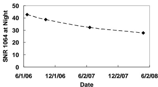
Fig. 5 SNR trend for the 1064 Channel at Night
