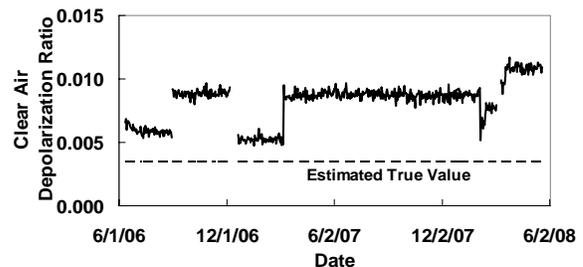
Fig. 11 Clear air depolarization ratio measurement trend
