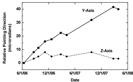
Fig. 7 History of the aligned pointing direction
