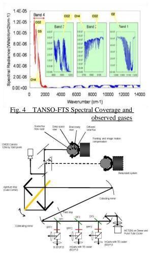
Fig.5 TANSO-FTS Optical Schematics
