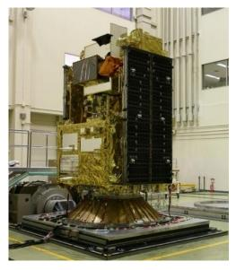
Fig. 2 GOSAT PFM under vibration test
