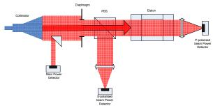
Fig. 2: Setup of transmission measurement
