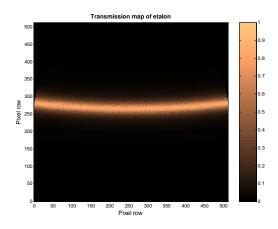
Fig. 1: Transmission map calculated with the MSP Fizeau etalon model including spherical bowing and roughness.
