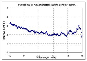
Fig. 6. Factor of improvement in transmission of a TeGeGaI fiber at liquid nitrogen compared to room temperature
