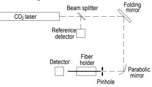
Fig. 3. Pulsed  $CO_2$  laser set-up for fiber attenuation measurements at 10.6  $\mu$ m
