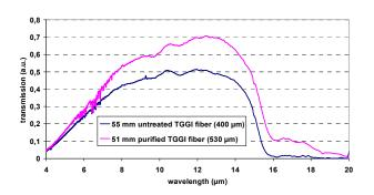
Fig. 4. Comparison of spectral transmission of a 5 cm fiber of purified and non-purified (untreated) TeGeGaI mono-index fiber
