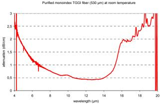
Fig. 5. Averaged spectral attenuation (dB/cm) of a purified TeGeGaI fiber at room temperature determined by fiber cut-back method
