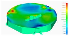
Fig. 4: Gravity effect from FEM analysis
