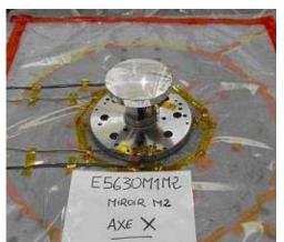
Fig. 9: M2 during vibration tests
