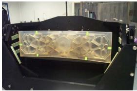
Fig. 7: M3 during interferometric test before coating
