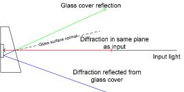
Fig. 7. Illustration of the light paths from the PMDG sample in the diffraction efficiency measurement.
