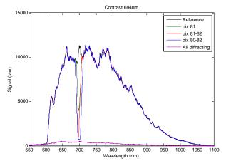
Fig. 13. Demonstrator modulation contrast with one, two and three pixels in diffracting state. The background signal in the all in a diffractive state is due to diffuse ghost reflection from the LVBF aperture.
