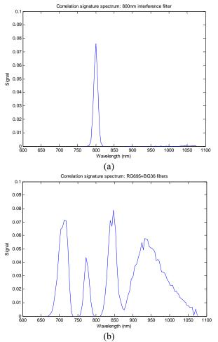
Fig. 16. Sample spectra for correlation signatures were taken from halogen lamp through a) 800 nm interference filter and b) RG695+BG36 filters. The signature means that the PMDG is programmed to reflect signal according to the measured transmission spectra.
