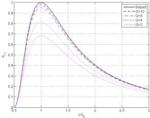
Fig. 2. Diffraction efficiencies of the order m=-1 for a staircase PMDG approximating the ideal blazed profile with Q levels and an ideal blazed profile.
