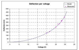
Fig. 5. Results of the model of deflection versus control voltage for the PMDG sample. In addition to the HeNe points, measurements were obtained from longer wavelengths.
