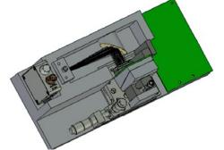
Fig. 12. Demonstrator opto-mechanical design. The PMDG sample is mounted on a tilt and translation platform.
