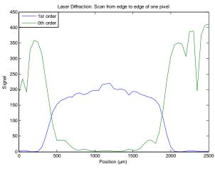
Fig. 6. The diffraction spot intensity from a scan along one pixel in diffractive state with 50  $\mu$ m steps. The signal in the 0<sup>th</sup> order is from outside the pixel structure
