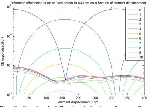
Fig. 8. Simulated diffraction behaviour for ten first orders for 633 nm. All the even orders are suppressed when the grating is in diffractive state but they do have a maximum with zero order when the displacement is 0 nm.
