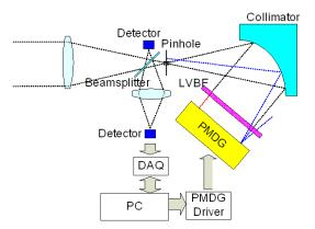
Fig. 10. A single-point miniature spectrometer. An onaxis concept with beam splitter, LVBF and PMDG.
