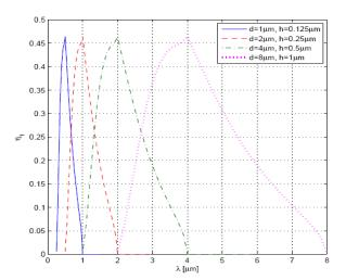
Fig. 1. Simulation of diffraction efficiency  $\eta_1$  for a hypothetical reconfigurable PMDG consisting of 0.5  $\mu$ m wide elements with different periods d and depths h.
