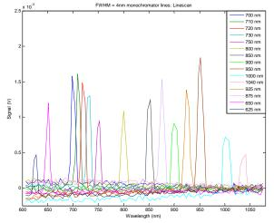
Fig. 14. Monochromator lines measured with the line scan method.
