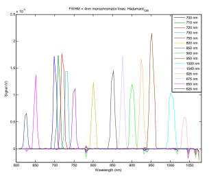
Fig. 15. Monochromator lines from HR640 measured with Hadamard method. The small spikes where multiple lines can be seen are caused by the drift.
