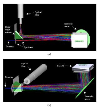
Fig. 11. Demonstrator optical design. (a) Side view. (b) Bottom view. Blue rays are accepted rays and green and red rays are rejected rays.
