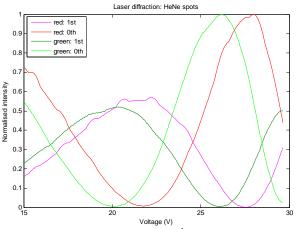
Fig. 4. Relative intensity of the 0<sup>th</sup> order (reflected) and 1<sup>st</sup> order spots versus control voltage.
