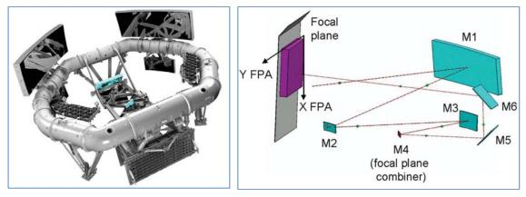
Figure 1: The GAIA Payload Module (PLM) with the two large M1 telescope mirrors on top (left; credits: ESA) and a schematic of the optical configuration
