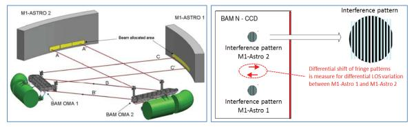
Figure 2: Schematic of Basic Angle Monitoring system with optical beams (left) and principle of fringe patterns on CCD (right).
