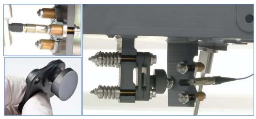
Figure 4: Cryogenic fiber collimator with the two dominating parts: fiber connector interface to SiC BAM structure (upper left) and the strongly curved off-axis parabolic SiC mirror.
