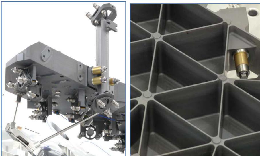
Figure 3: Details of SiC BAM OMA bar 2 with optics, periscope and Invar iso-static mount (left) and open backside structure of SiC baseplate (right).
