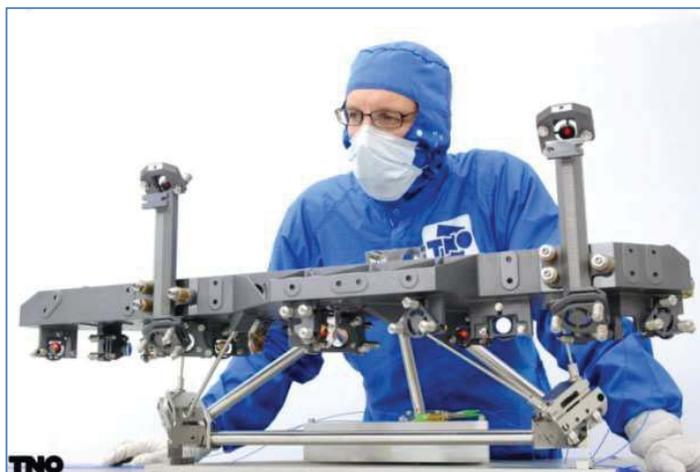
Figure 6: Thermal testing of GAIA BAM on Invar set-up.
