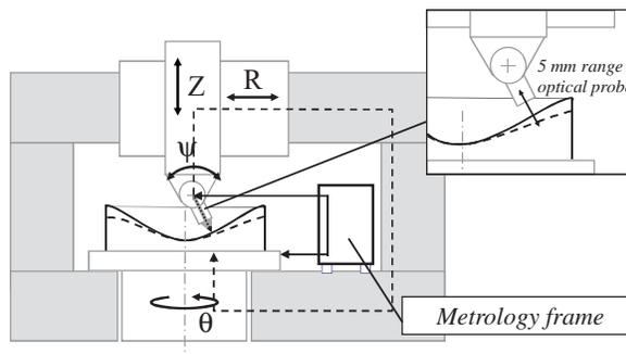
Figure 6. NANOMEFOS machine concept with long range optical probe and separate metrology frame
