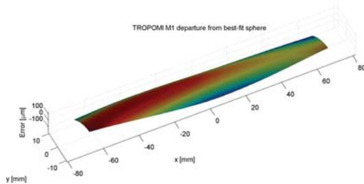
Figure 4. Deviation of nominal primary mirror surface with best fit conic
