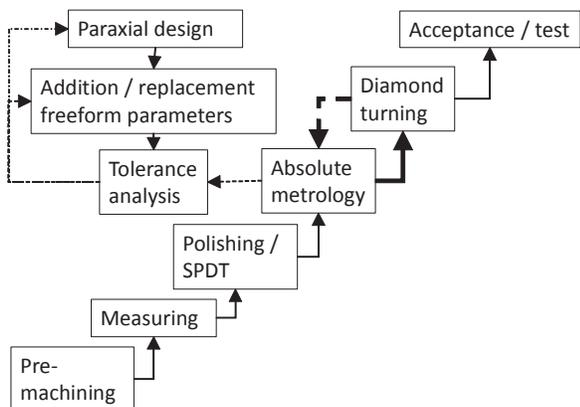
Figure 1. Freeform manufacturing value chain. The bold arrows indicate an iterative loop
