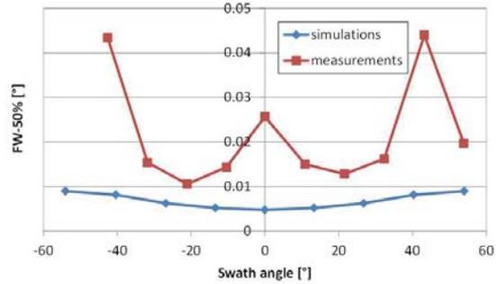
Figure 10. Resolution (FW-50%) of breadboard telescope measurement and simulation
