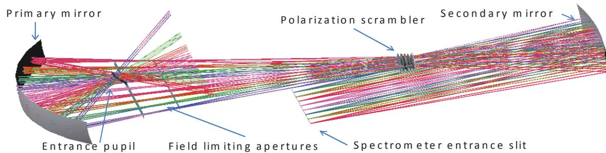
Figure 3. 3D view of TROPOMI telescope
