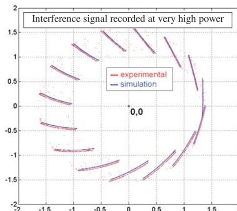
Figure 10. Spikes recorded at very high power, for different position of the target: complex plane representation. The optical frequency is kept constant. Blue data: simulation, with  $\varepsilon = 0.22$ , taking into account the AM-to-PM and saturation effects
