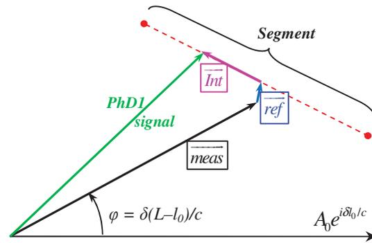
Figure 2. Addition, in the complex plane, of the three contributions to the PhD1 two-mode interference, signal. The phase  $e^{i\delta_0/c}$ , of the PhD0 photodiode, is taken as the phase reference.
