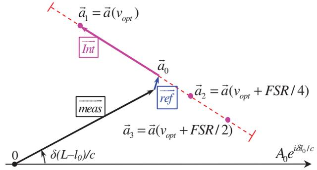
Figure 4. The three data points: choice of the sequence of three different optical frequencies
