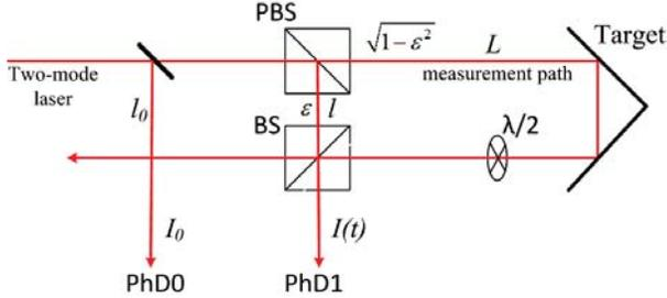
Figure 1. Schematic diagram of the telemeter
