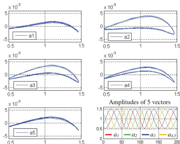
Figure 8. Segments obtained with 60000 5-fold data groups, when the master laser is slowly scanned (about 200 MHz in 5 minutes). These recordings are performed with a path length  $L$  such that the segment is radial, that is, the situation where the change in the signal amplitude, and hence the AM-to-PM effects are maximum. As in Fig. 7, the transverse coordinate is magnified, to highlight the distortions.
