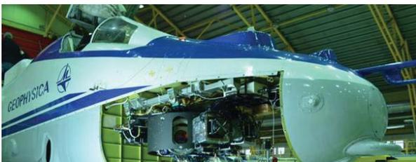
Fig 1: GLORIA mounted in bay no. 1 of Geophysica M55
