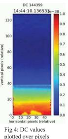
The interferogram's maximum position represents the static shear. The static shear was adjusted on-ground before takeoff. The plot was done with a dataset measured during flight where the temperature of the interferometer drifted from the initial value by 15 K. A very small maximum shear of +/-1 micrometer has been determined.
