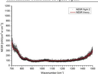
Fig 7: Chemistry mode NESR plot. Black dots represent the measurement and the red line the theoretical expectation.
