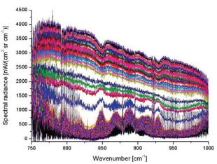
Fig 6: Chemistry mode calibrated spectra in the range of 750  $\text{cm}^{-1}$  – 1400  $\text{cm}^{-1}$ , 128 (v) spectra are plotted; these spectra are the mean of the 48 (h) pixels.
