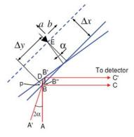
Figure 2: Schematic representation of the influence of alignment and jitter parameters of the mirror on the optical path delay of the incoming laser beam.
