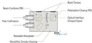
Figure 7: The chosen Fiber Switching Unit Concept.
