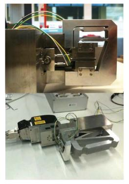
Figure 13: Picture of the piezo-stepper test set-up, to measure the errors during constant velocity motion, introduced by stepping.
