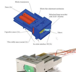
Figure 1. Top: CAD design of the Point-Ahead Angle Mechanism as designed by TNO Optomechatronics, including all its components. Bottom: Realization of the Point-Ahead Angle Mechanism. The mirrors can be actuated by one of two piezo-stacks. The mirror is mounted with a bonded iso static mount design for details see [6].
