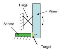
Figure 4: Schematic illustration of the active target capacitive sensor. The sensor measures the displacement of the tip of the mirror. The tilting of the mirror is taken into account by one-time calibration.
