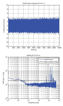
Figure 14: Top: Time domain result of the tracking error of the piezostepper set-up during 10000 seconds of 0.5 nm/s motion. Bottom: Amplitude spectral density of the tracking error of the piezostepper set-up, during 10000 seconds of 0.5 nm/s motion.
