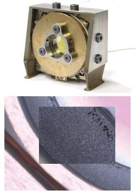
Figure 12: Top: The FSUA with integrated angular measurement system. Bottom: a photo of one of the sliding contact surfaces after the life test no signification degradation of the surface.
