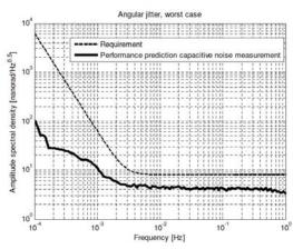
Figure 5: Performance prediction of the angular jitter, based on capacitive noise measurements under controlled environmental conditions. A dynamical model of the PAAM and the controller is included. The predicted performance is below specification.
