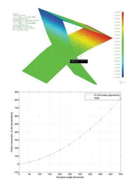
Figure 3: Top: Meshed FEM model of the Haberland hinge, actuated to an extreme angle. Outcome of the FEM analysis is the longitudinal and lateral jitter of the axis of rotation. Production tolerances of  $\pm 10$  µm are taken into account. Bottom: The piston movement of the axis of rotation under different actuation angles. By taking the derivative of the fitted polynomial, the piston sensitivity can be determined for different angles.
