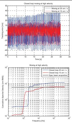
Figure 15: Top: Time domain result of the tracking error of the piezostepper set-up during 30 seconds of 10 and 20  $\mu$ m/s motion. Bottom: Cumulative Spectral Density of the tracking error of the piezostepper set-up during 30 seconds of 10 and 20  $\mu$ m/s motion.
