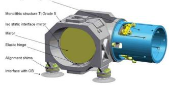
Figure 16: CAD picture of the IFPM beam steering mirror design, including redundant piezo steppers.
