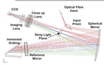
Figure 9: Test setup for stray light measurements
