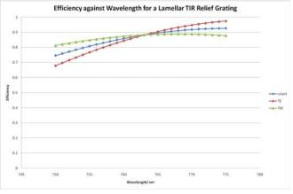
Figure 7: Immersed Grating theoretical efficiencies
