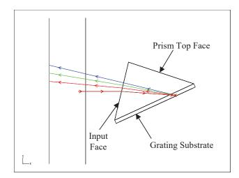
Figure 4: Ray trace in an Immersed Grating
