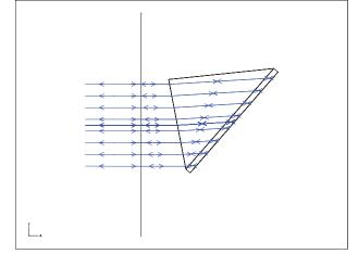
Figure 5: Littrow condition used for interferometric tests
