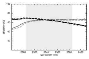
Figure 5 FM grating efficiency with TM polarization in Grey and TE polarization in black. Simulated data are dashed, measured data continuous.
