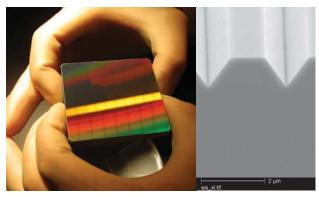
Figure 3 Left: The FM immersed grating during final inspection. Right: Scanning electron micrograph of V-groove grating profile on a test piece.
