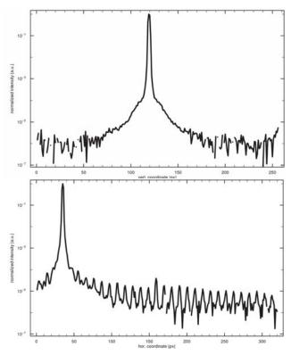
Figure 4 FM grating stray light, in across-spectral direction (Top) and in spectral direction (Bottom). The regular array of peaks at the 10<sup>-5</sup> level stems from laser side-modes, the actual stray-light level is 10<sup>-6</sup>.
