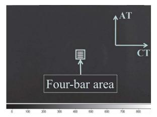
Fig. 9. Image of four-bar target as captured by CIRC for evaluation MTF
