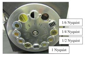
Fig. 8. Four-bar targets mounted on the collimator system
