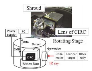
Fig. 6. Schematic view of MTF measurement
