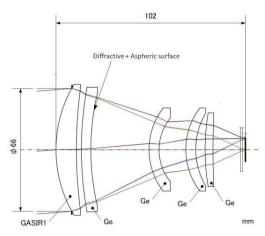
Fig. 5. Optical design of the CIRC
