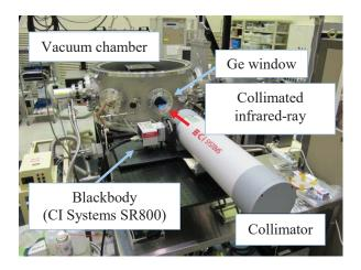
Fig. 7. Experimental setup of MTF measurement
