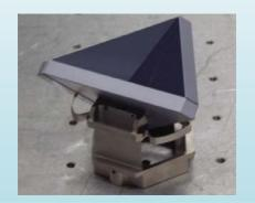
Three triangular silicon mirrors assembled by irreversible molecular adherence onto a MFD
