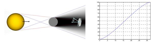
Fig. 3. LEFT: Shadow and penumbra pattern projected behind the occulting disk. The arrows show the possible off-pointing  $(\theta')$  of the Coronagraph-S/C. **RIGHT**: Profile distribution of the illumination in the penumbra at 150 m beyond the occulting disk. The x-axis is the angle between the Sun-axis and the Formation Axis in arcmins; the y-axis is the %. of the received Solar intensity.
