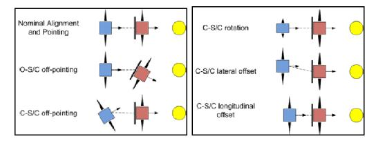
**Fig. 2.** All possible displacements/misalignments of the two spacecrafts. The satellite on the left is the Coronagraph-S/C (C-S/C), while the satellite facing the Sun (circle) is the Occulter-S/C (O-S/C).
