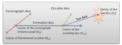
Fig. 1. Definition of the different axes of the system. Proc. of SPIE Vol. 10565 105652S-2
