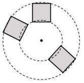
Fig. 6. Circular symmetry around the Sun axis. Both SPS and OPS are not able to determine the orientation of the formation around the Sun axis.
