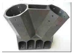
Figure III-8 view of the Si<sub>3</sub>N<sub>4</sub> end-fitting part
