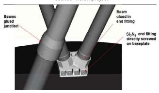
Figure I-2 Full  $Si_3N_4$  junction allowing a direct connection of the truss to the instrument baseplate
