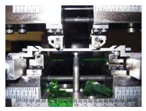
Figure III-1 4 pt bending test set up on large samples
