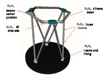
Figure I-1 Example of a 2 meter telescope Si<sub>3</sub>N<sub>4</sub> truss structure designed for Euclid telescope in the frame of ESA cosmic vision project
