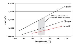
Figure II-1Coefficient of thermal expansion CTE for structural "optical" materials
