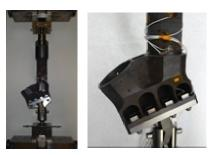
Figure III-9 beam end fitting junction tensile test and view of the screwed end fitting on the I/F plate
