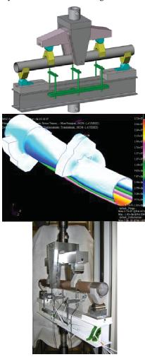
Figure III-2 bending tests up rupture including FEM comparison and rupture mode
