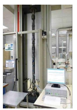
Figure III-7 2meter joined beams tested in tensile
