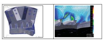
Figure III-11 A unflatness of 30µm at I/F generate 50 Mpa stress increase
