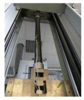
Figure IV-1 Tensile proof test on flight beam
