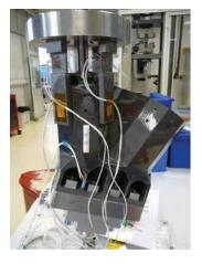
Figure IV-2Proof test on the flight end fitting
