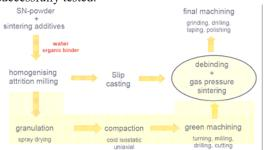
Table II-2 production process for silicon nitride lightweight component
