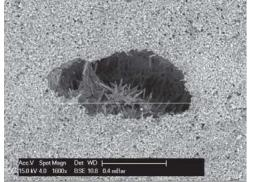
Figure V-1 : residual porosity found on the tested samples
