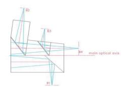
Figure 3. Light splitted in the Prism
