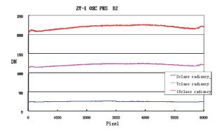
Figure 11. Response curve of B2 band at different radiance
