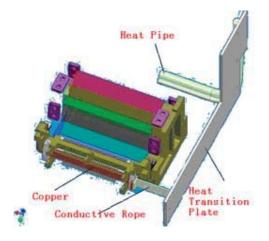
Figure 9. The dissipation chain of the CCD
