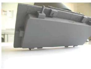
Fig. 2. Mirror blank after CVD cladding
