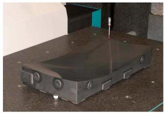
Fig. 4. CMM measurement on M3 mirror
