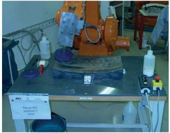
Fig. 3. Robot lapping of M3 mirror
